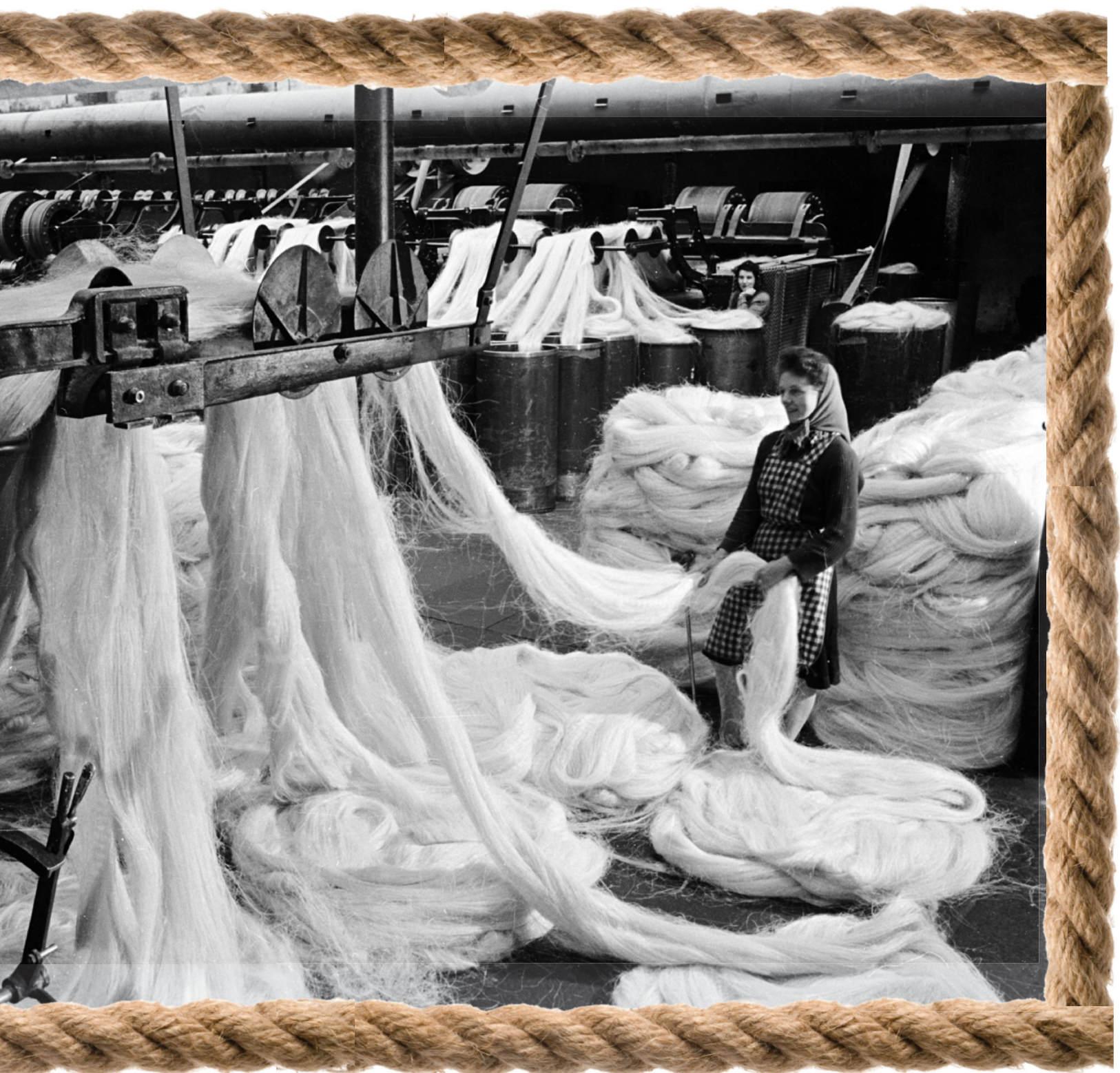
Spinning around: hemp fibre prepared for spinning at Gourock Ropeworks, Port Glasgow, in 1946—now, the crop is making a comeback
